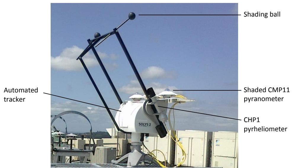
Figure 1.7: UKZN HC ground station with first class pyrheliometer and secondary standard pyranometers.
