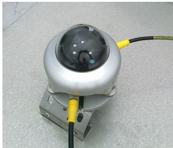
Figure 1.8: A Delta-T Devices Ltd. SPN1 radiometer installed at the UKZN Howard College ground station.
